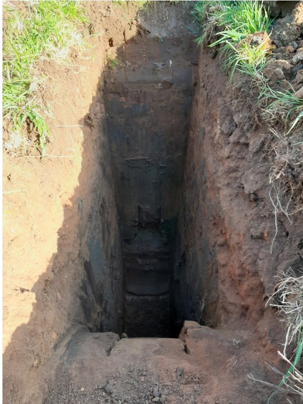
Photograph 9: TP04, dug from the top of the embankment platform.
